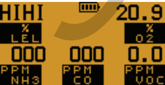
Display in alarm conditions
